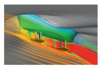
Hull and propeller optimized by state-of-the-art CFD methods to eliminate interaction effects between bow and stern VSP and ensure safe and efficient operation in 360°.
