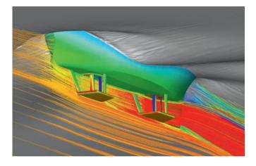
Hull and propeller optimized by state-of-the-art CFD methods to eliminate interaction effects between bow and stern VSP and ensure safe and efficient operation in 360°.
