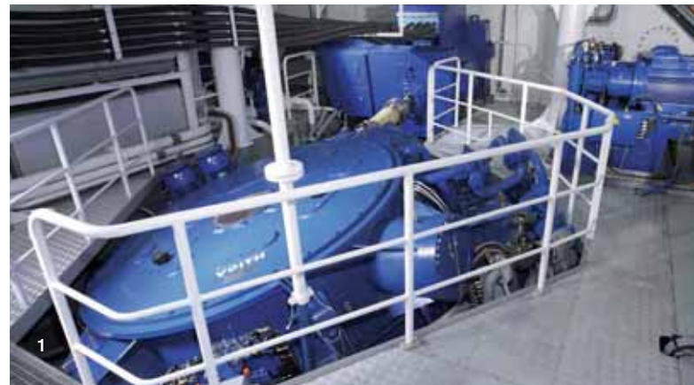
2 Bow arrangement of two VSPs
