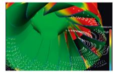
Voith aerating runner: blade discharge edge slots allow for maximum bubble distribution
