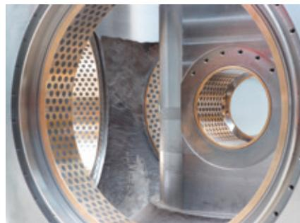
Advanced technology for Castrelo hydropower plant in Spain: oil-free hub.
