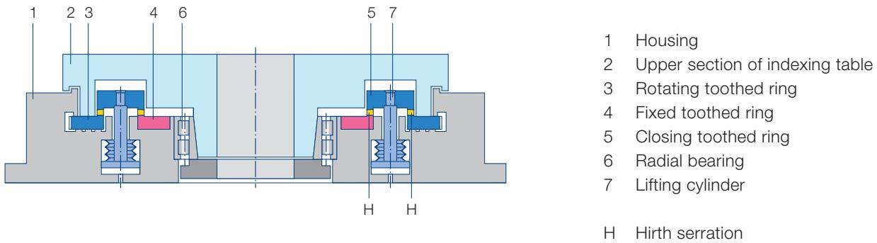
Schematic diagram of non-lifting rotary indexing table with Voith Hirth serration in 3 toothed ring design
