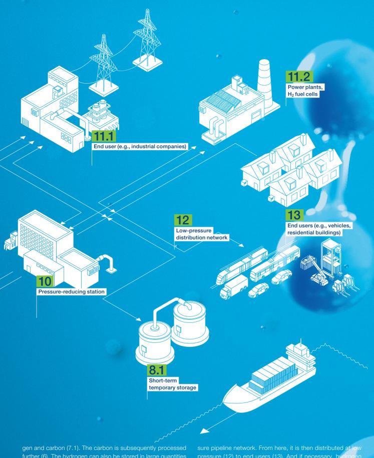
gen and carbon (7.1). The carbon is subsequently processed further (6). The hydrogen can also be stored in large quantities until it is needed (8.1, 8.2). Distribution (9) to decentralized pressure-reducing stations (10) takes place via a high-pres-
