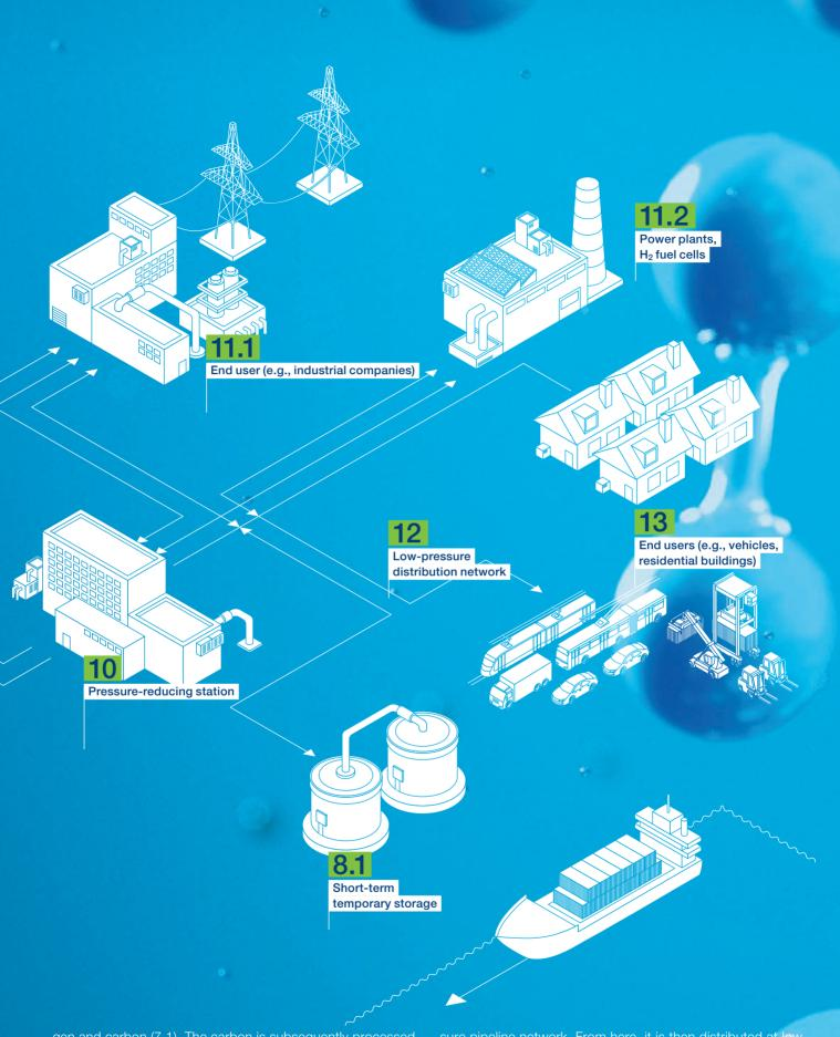
gen and carbon (7.1). The carbon is subsequently processed further (6). The hydrogen can also be stored in large quantities until it is needed (8.1, 8.2). Distribution (9) to decentralized pressure-reducing stations (10) takes place via a high-pressure pipeline network. From here, it is then distributed at low pressure (12) to end users (13). And if necessary, hydrogen can also be converted directly back into electricity in power plants (11).
