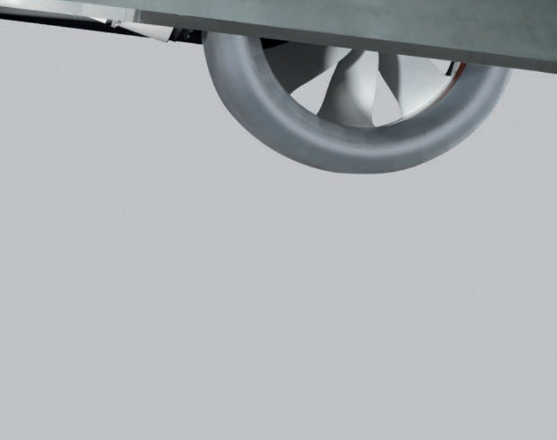
Voith Inline Propulsor in swing out /azimuthing configuration
