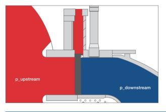
There is a strong suction peak at the bottom as the ring gate closes. The design and precise position of the seal prevents leakage and unintentional opening.
