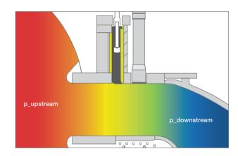
The ring gate is lowered through its housing by the electronically controlled servomotors. The pressures above and below the ring gate must be equalized.
