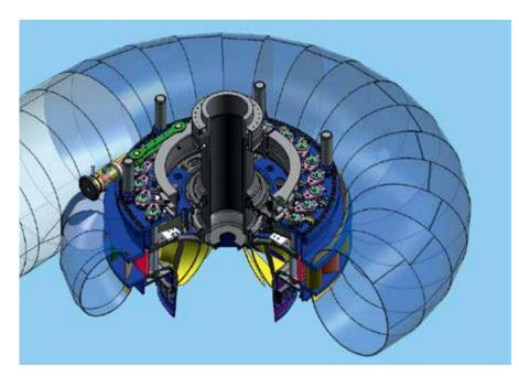
Ring gates (here in red) provide a useful addition for large Francis turbines, where a spherical or butterfly valve would be too large.
