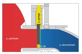
The pressure in the ring gate housing (garage) is determined by the design and size of the gaps (deliberate control of the pressure differentials through leakage flow regulation).
