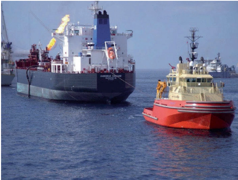
Figure 1: Voith Water Tractor, Forte , equipped with two Voith Schneider Propellers (VSP36EC) and the electronic Voith Roll Stabilization (VRS)
