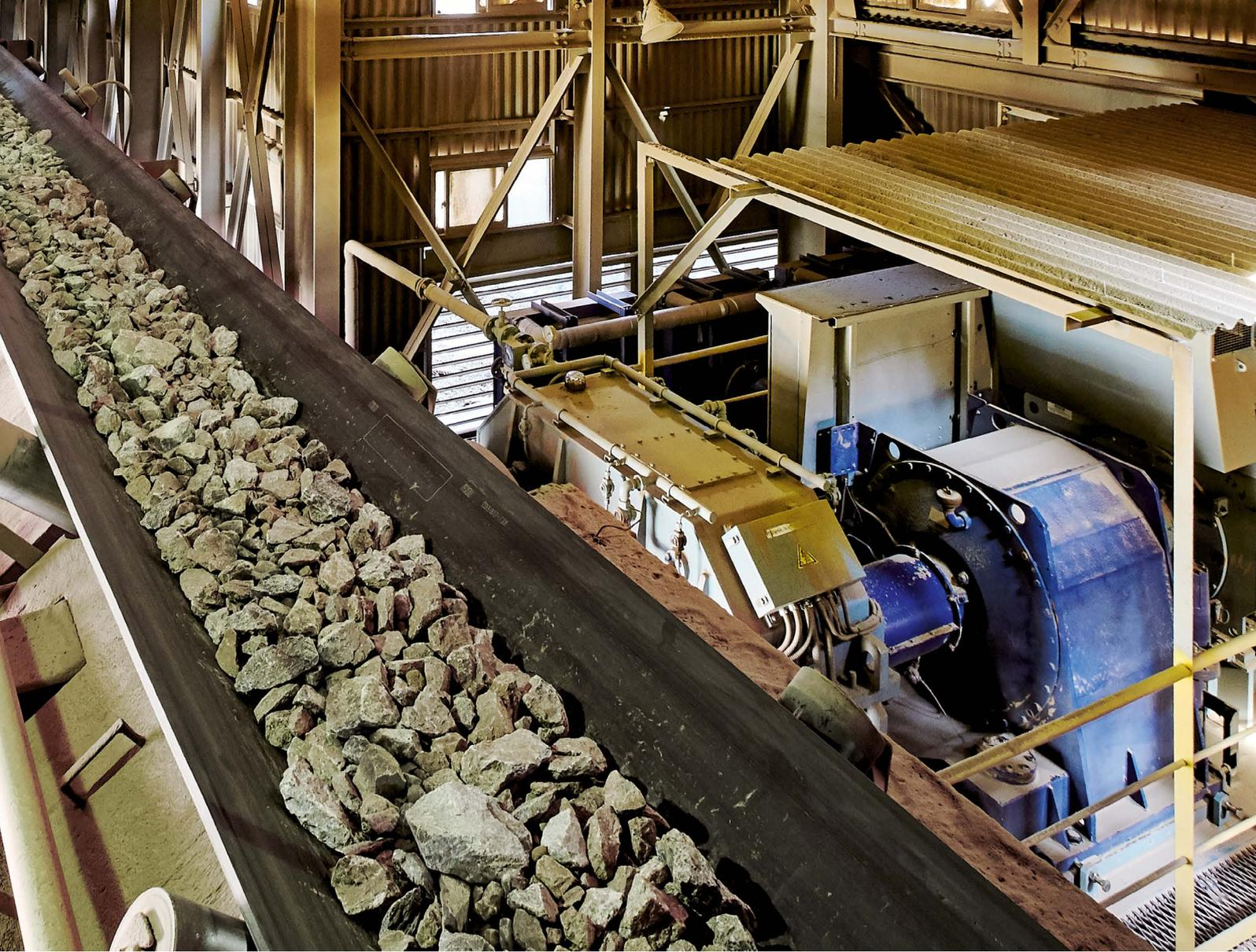
**Voith provides turnkey solutions with complete packaging, including the integrated controls. For remote service purposes the drive units can be equipped with vibration sensors and other condition monitoring intelligence.**
