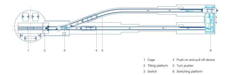
With Voith TurboHoist Decking Devices, high safety standards prevail in mine car operation thanks to guided and pre-defined movements of the mine cars, controlled and limited speed, and safety devices prior to accessing the shaft area. Our products allow moving the wagons in a safe, reliable and precise way in the area of the shaft as well as onto and off the hoist. Furthermore, the system permits safe passage for mine personnel onto and off the hoist.
