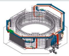
The highest amount of cooling water is nevertheless used up by the generator. For this reason the innovation of the ,Cooling on Demand' principle begins here.
