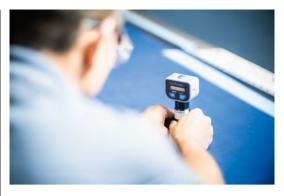
**Precise Inspection**A Voith employee measures the hardness of a shoe press sleeve.
