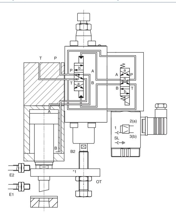
Proximity switch E1 and E2 and the mechanical parts  $^{\star}1$  are not scope of delivery.
