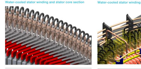
In water-cooled generators, the losses originated in the generator stator winding, the stator circuit rings, the phase connectors as well as some stator core losses are not only dissipated by the traditional air-coolers but also through a direct water cooling.
