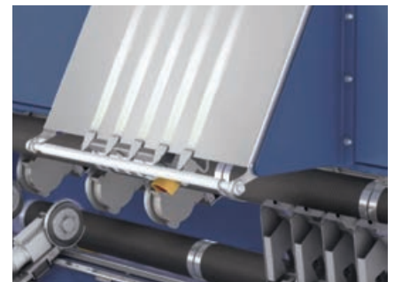
Air nozzles and transfer tables
