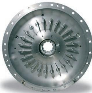
Adjustable guide vanes can be controlled by a pneumatic, hydraulic or electric actuator, which receives an input signal of 4 to 20 mA or 0.2 to 1 bar from the customer’s master control system. The feedback signal, to incorporate the torque converter in a closed control loop, can be provided by switches or as a 4 to 20 mA signal.
