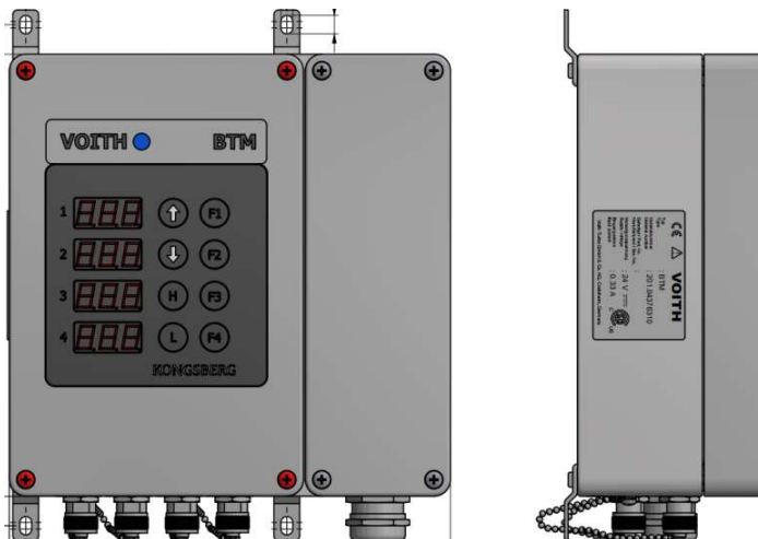
Picture 3: Exemplary image of the new, all parametrized version of the SPU incl. blue marking
