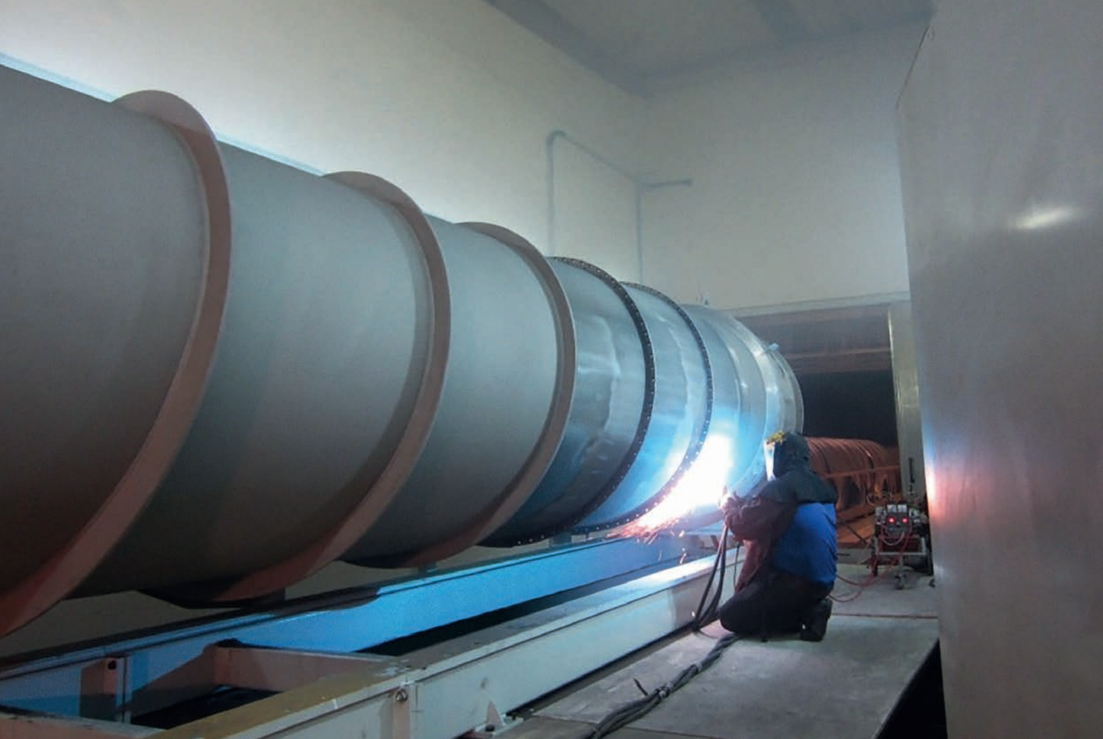
Refurbishment of a press screw in a Voith workshop
