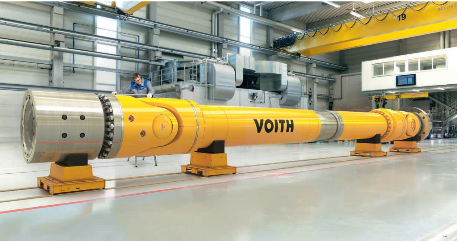
High-performance universal joint shafts in the assembly hall; E joint (left)
