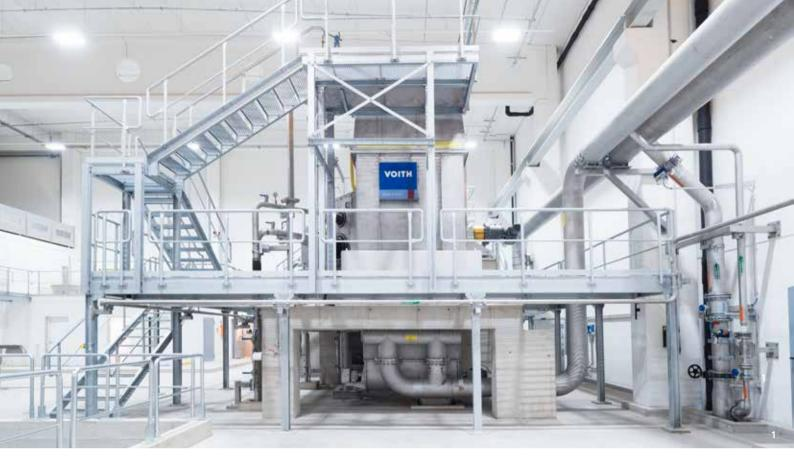
Continuous filtrate quality over a long period as well as low operation and maintenance costs are essential for a reliable and efficient dewatering process. However, fiber suspension thickening inside the vat can lead to mechanical stresses and damage to the discs. As a result, typical filters operate with limited inlet consistencies. This requires significant pumping of dilution water and the use of filters sized for a high volumetric load.
