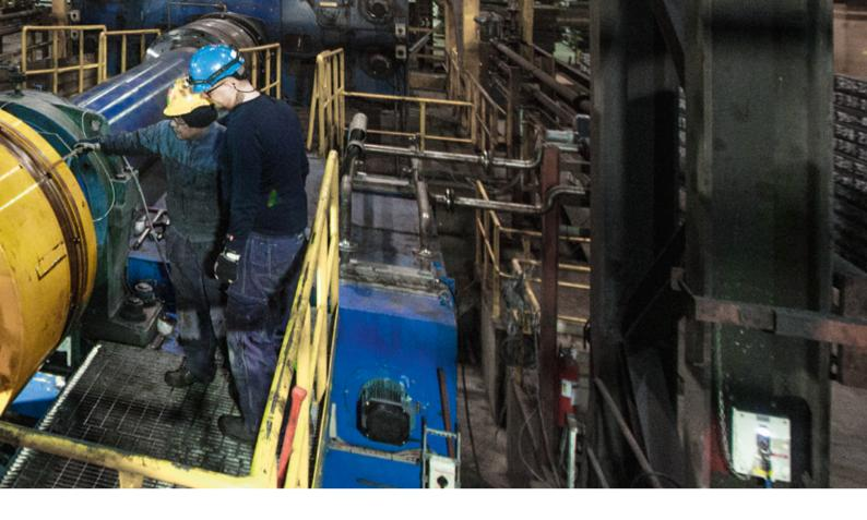
At Voith's site in Hudiksvall, 400 kilometers north of Oxelösund, worn couplings are repaired and made fit for reuse. Two SafeSet torque limiting couplings are currently in use in Oxelösund. To ensure downtimes are as short as possible in the event of overload, SSAB keeps one spare SafeSet coupling in stock.
