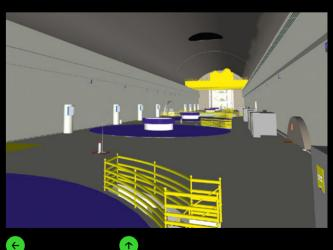
One of the four turbines in Paulo Afonso. The 3D model of the powerhouse helps to visualize the specific spatial conditions in the power plant.
