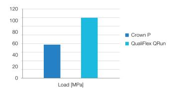
QualiFlex QRun has a low crack propagation.
