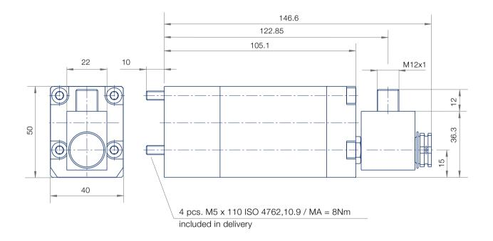
All dimensions are in mm Solenoid free rotatable
