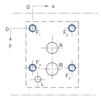
F: M5, thread depth min. 12 mm All dimensions  $\pm$  0,1 mm
