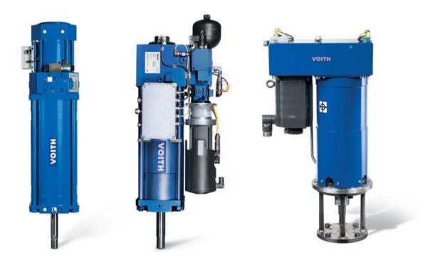
A trip actuator is a linear on/off actuator, which is mounted to the trip valve and actuates it directly. The drive solution is compact and forms a complete unit. We offer three different trip actuators: electrohydraulic, self-contained electrohydraulic and electromechanical drives.
