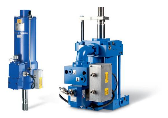
A control servo motor is a linear, electrohydraulic actuator. It is mounted to the control valve and actuates it directly. The control variable is the stroke s of the piston rod. The rod position feedback is integrated into the servo motor. Control servo motors are available with single-acting or double-acting cylinders. Various components of the servo motors may have redundant design.
