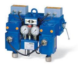
An I/H converter module is a completely redundant system with two I/H converters connected in parallel (hot redundancy). Electronic fault detection is integrated. In the event of a I/H converter failing, the function is ensured by a hydraulic maximum selection.
