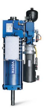
A SelCon self-contained actuator is a linear, electrohydraulic drive without external oil supply. It is mounted to the control valve and actuates it directly. The control variable is the stroke s of the piston rod. The rod position feedback is integrated into the drive. The self-contained hydraulic system is also integrated into the drive.
