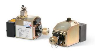
An I/H converter is a current-to-pressure converter. It regulates the pilot valve of a hydraulic cylinder that actuates the control valve. The hydraulic pressure p is the control variable. The position of the piston rod is generally fed back mechanically to the pilot valve. This is a simple, reliable and cost-effective solution.
