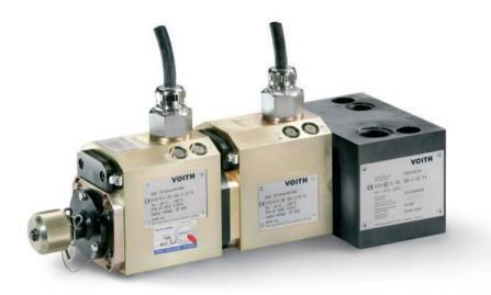
A tandem way valve is a way valve with two control magnets. These control magnets are connected in series and form a redundant unit (warm redundancy). If one control magnet malfunctions, the other takes over the control task. The switching logic is located in the distributed control system (DCS) and monitors the control magnets.
