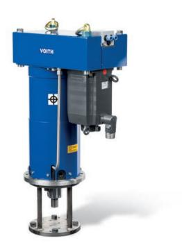
The EMA electromechanical actuator is a linear and oil-free actuator. It is mounted to the control valve and actuates it directly. The control variable is the stroke s of the actuator spindle. The spindle position feedback is integrated into the drive.
