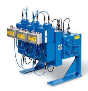
A trip block is an electrohydraulic safety control unit. It directly regulates the hydraulic cylinder that actuates the trip valve. The structure is triple modular redundant with a 2-out-of-3 voting (2003). A high flow rate allows very short trip times. All the solenoid valves can be isolated from the hydraulic system.
