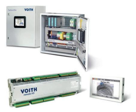
Standard controllers have a modular design with industry-proven hardware. The software is "pre-engineered" and the operation of the user interface is intuitive. After connection and configuration, the standard controllers are ready for operation. Integration into a distributed control system (DCS) is easy with various communication interfaces. A 7" TFT LCD control panel with touchscreen interface is used for operation.
