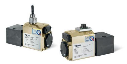
A CTo detects overspeed and directly controls the hydraulic cylinder that actuates the trip valve. The assembly is compact and has short signal paths. It is usually mounted directly on the hydraulic cylinder for the trip valve.
