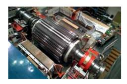
Motor-generator Usually high-speed machines, air- or water-cooled, operable with reversible pump-turbines or in ternary sets. > Output: approx. 530 MVA; Voltage: up to 23 kV
