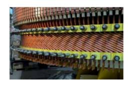
Asynchronous generator Air-cooled, usually vertically installed, and also used as motor-generators. Suitable for variable-speed pumped-storage, though rarely installed. > Output: up to 500 MVA; Voltage: up to 22 kV
