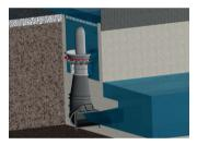
The vertical arrangement of the turbine with rotatable suction pipe permits a change of direction for the water flow. The result is a high degree of flexibility, when replacing turbines in existing systems.
