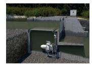
Because it routes the water through a shaft and a horizontal trash rack with underwater trash rack cleaning machine, the shaft power plant is short and compact. This significantly reduces the civil construction costs.
