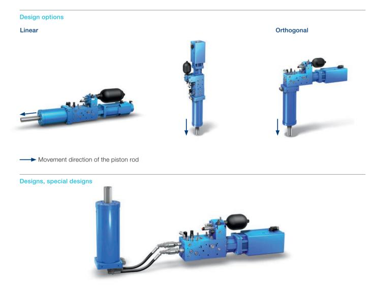
The special split design has been developed for use in very cramped installation situations. The pump group and the servomotor form a unit and the cylinder forms its own unit. The units are hydraulically connected by pipes or hoses. The split version offers extended design options compared to the standard series. All advantages of the CLDP are preserved.
